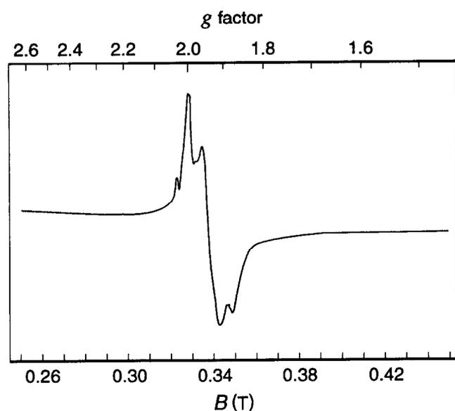
Fig. 1. EPR-spectrum of the reduced *M. barkeri* ferredoxin. The protein (0.66 mg/ml) was reduced with 2 mM dithionite and frozen in liquid nitrogen. EPR conditions: microwave frequency, 9.1799 GHz; modulation frequency, 100 kHz; modulation amplitude, 2 mT; microwave power, 3.2 mW; temperature, 13 K.
